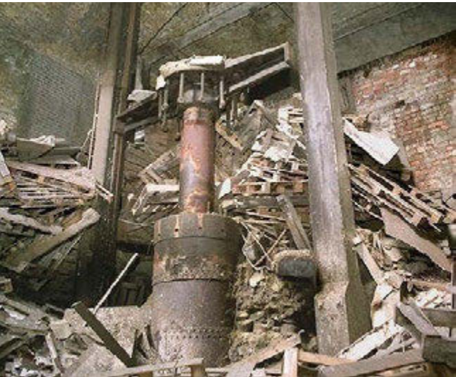
Fig 4.10.2: The hydraulic accumulator
